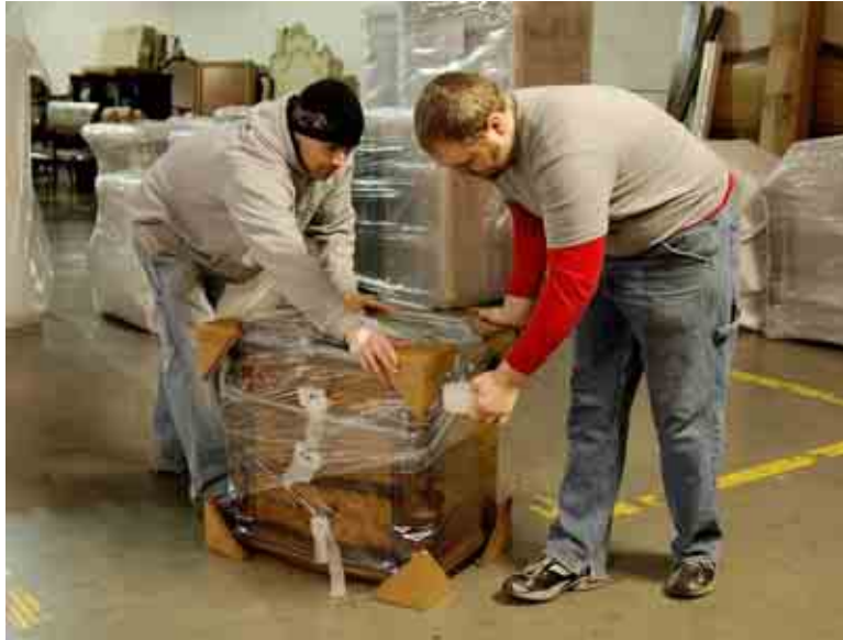
photo: edge protection applied
