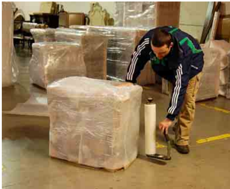
photo: over-layer of cellophane shrink-wrap
